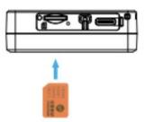
The locator is facing up The chip of the card is facing down and the card notch is facing the locator
