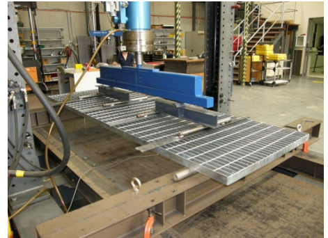
FIG.2 G505/40/100 TEST SET-UP
