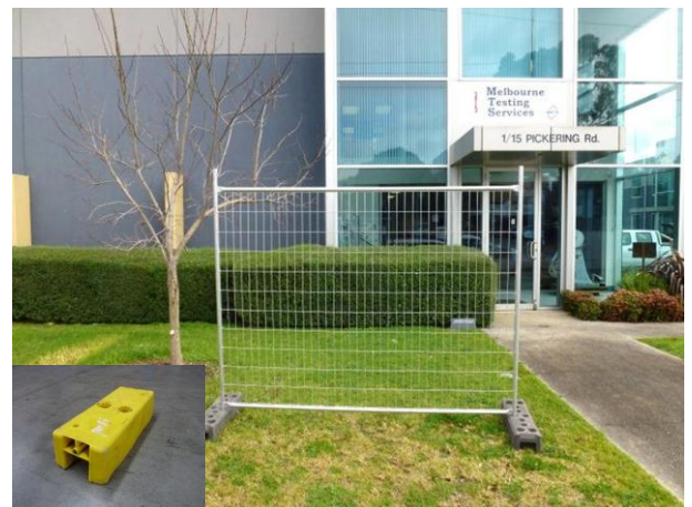
FIG.1 FENCE TEST PANEL SET-UP (INSET CONCRETE FOOT BLOCK)
