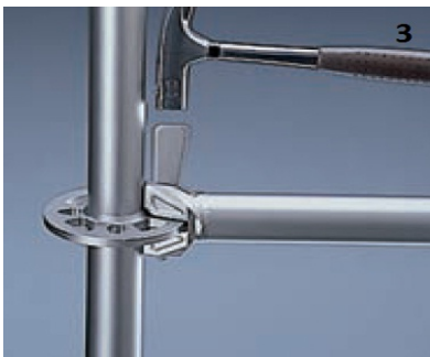
A hammer blow on the wedge transform the positive connection into a non-positive one.
